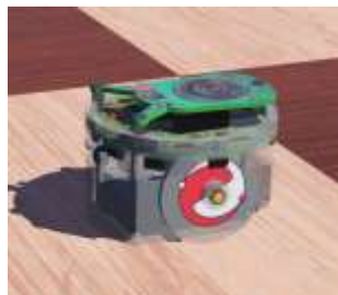
Figure 3. The e-puck mobile robot model in Webots
